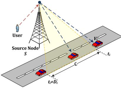
Fig. 1. Source-Vehicle communication in a two-hop VDTN.
