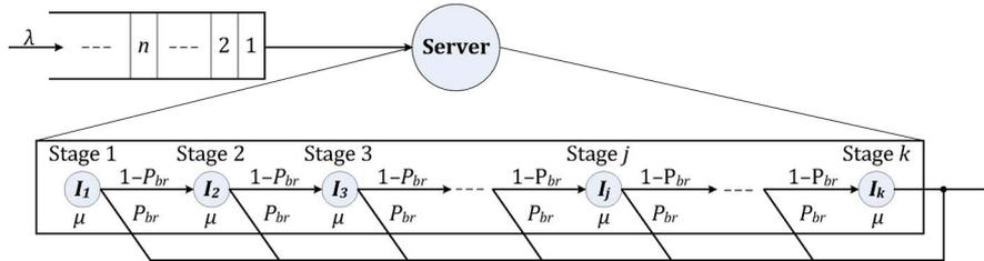
Fig. 4. Bundle service time composed of several waiting stages.
