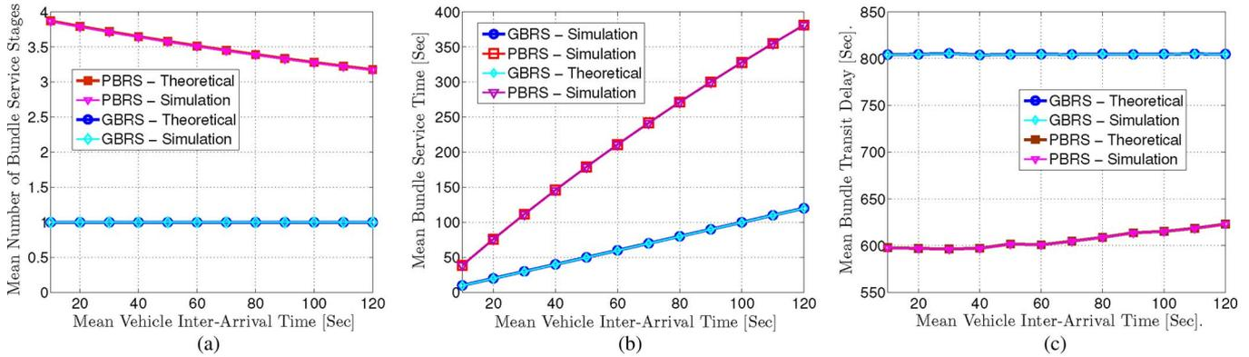
Fig. 5. Theoretical and simulated performance evaluation of the PBRs and the GBRS. (a) Mean number of service stages. (b) Mean bundle service time (in seconds). (c) Mean bundle transit delay (in seconds).
