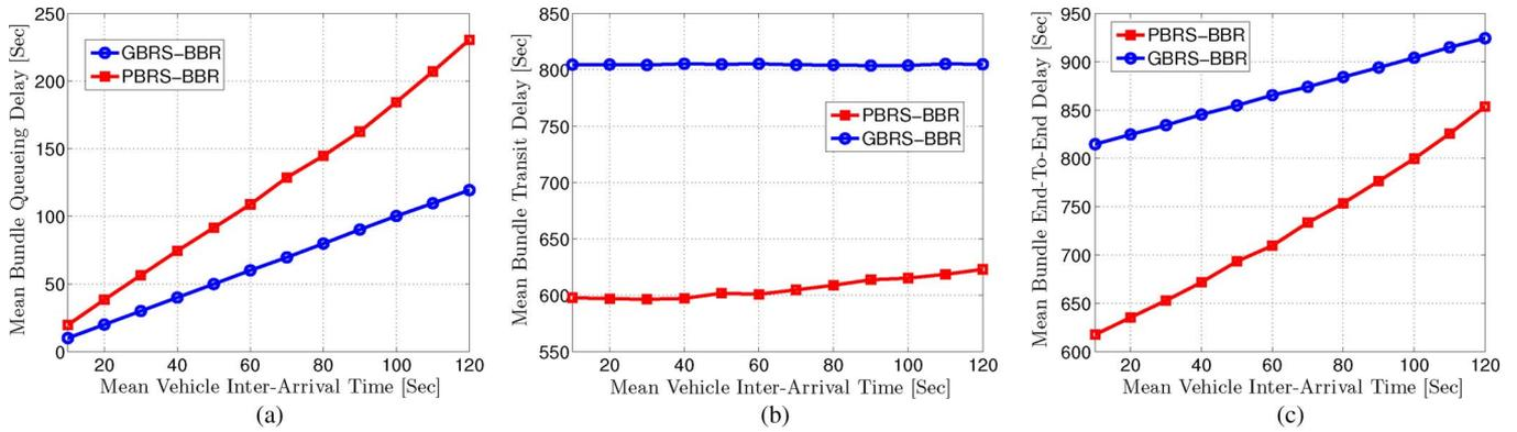
Fig. 7. Delay Performance of the PBRs-BBR versus the GBRS-BBR. (a) Mean queueing delay (in seconds). (b) Mean transit delay (in seconds). (c) Mean end-to-end delay (in seconds).
