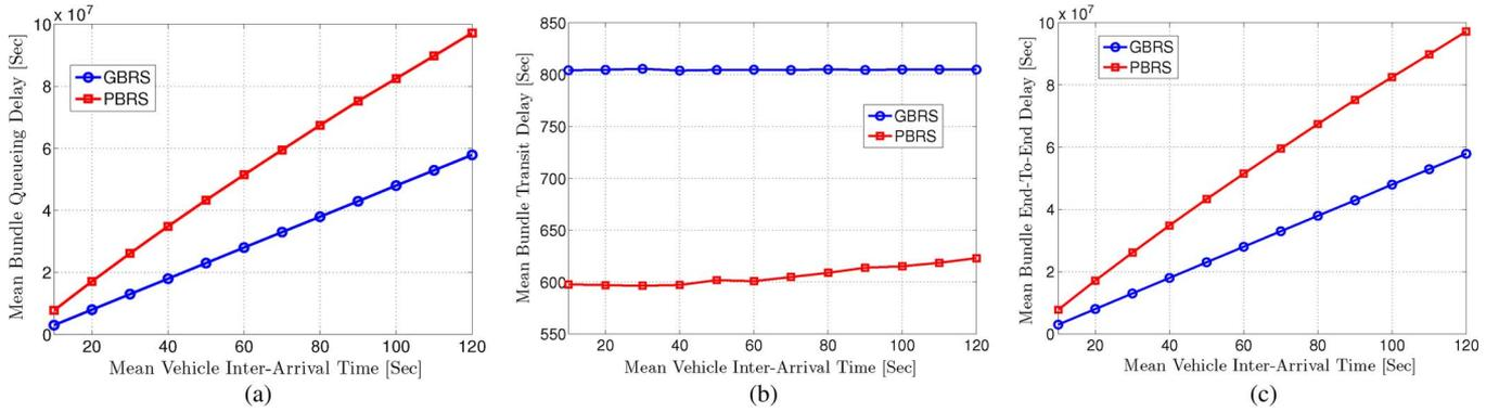
Fig. 6. Delay Performance of the PBRS versus the GBRS. (a) Mean Queueing Delay (in seconds). (b) Mean transit delay (in seconds). (c) Mean end-to-end delay (in seconds).
