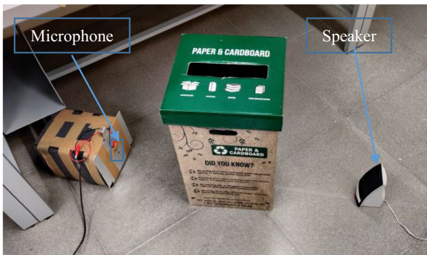
Fig. 20 A cardboard obstacle placed in the middle of the path between the speaker and microphone
