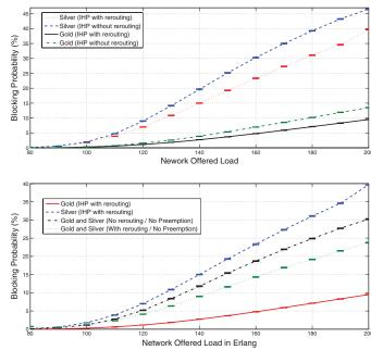
Fig. 3. IHP with/without rerouting setup strategies (uppermost); IHP with rerouting strategy vs. traditional setup schemes (bottom).
